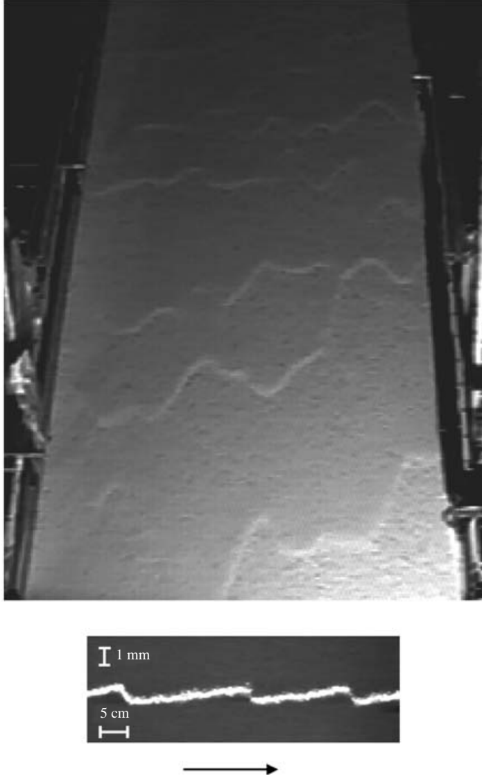
FIGURE 1. Free surface of sand flow showing the long surface waves. Material is flowing downwards; the plane width is 70 cm. Shown below is a typical thickness profile of the natural waves measured with a laser sheet light (see Pouliquen 1999 a for description of the method). The arrow gives the flow direction (sand 0.8 mm in diameter, \theta = 34^\circ , h = 4.6 mm).
